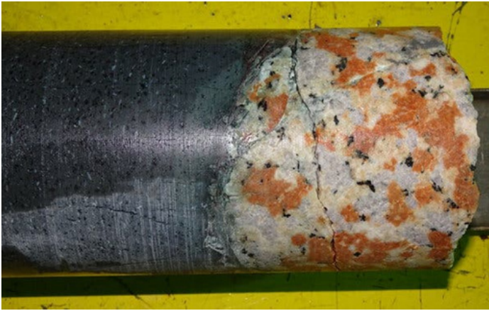
Figure 7. Drill Core from the Chicxulub Peak Ring. Seen here is a visible transition at a depth of ~700 meters. The pink and white composite granite on the right, originating in basement levels of the Earth's crust, was splashed up as liquified rock, then washed outward to form the foundational material of the peak ring. During rebound, molten rock washed back over the peak ring, burying it under 40 meters of breccia and suevite, seen to the left. More then poured into the crater. Subsequently, tsunami backwash added layers of sand, gravel, and charred floral remains that were swept into the crater from distant beaches and burning forests. Source: See Smith.
