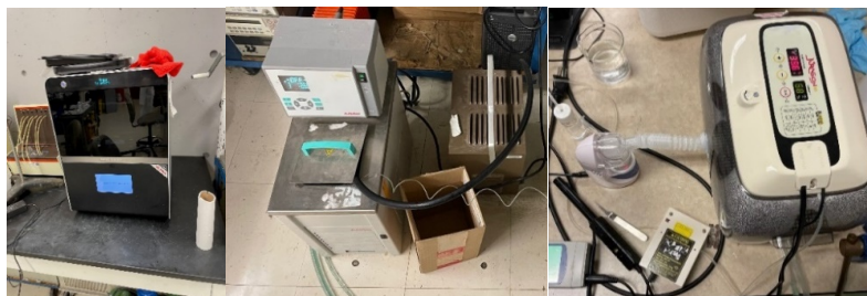
Figure 4: Equipment used for physical trials of each surface. From left to right: MiiCraft Ultra 150 DLP Printer, Julabo HE Circulator, U-Cool external chiller, Ultrasonic Nebulizer, and incubator with small vial of distilled water and pump to maintain humidity. A beaker of distilled water is kept on hand to refill humidity generating components.
